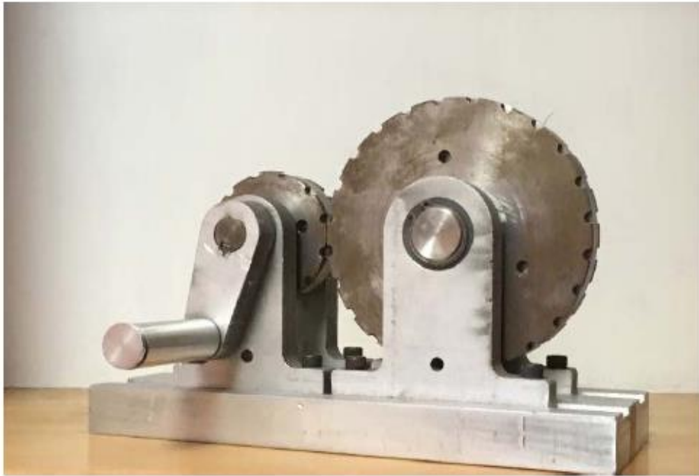
Figure 7.4 Demonstration unit of transmission having only one ring magnet
