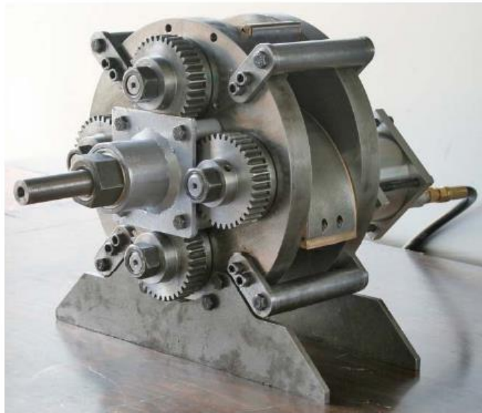
Figure 5.12 Engine with reciprocating admission valve and full set of seals
